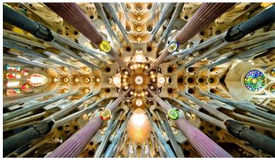
As for the structure of the church, it is remarkable for its height and its lightness. It is revolutionary in terms of the building resources used, which characterise **Gaudí**'s entire life's work: the catenary arch, sloping columns and hyperboloid vaults. **Gaudí** passed away in 1923 without having been able to complete the construction, but various architects have planned and keep working to finish it following the documents left by the genius.
